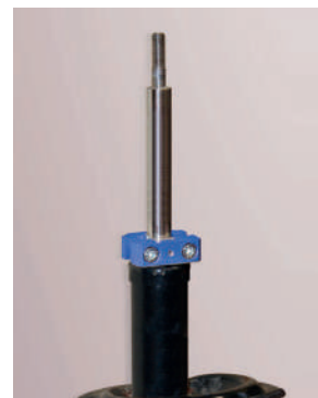
Remove the rod-puller after locking the clamp in its final configuration. Mount the spring and remove the clamp.
