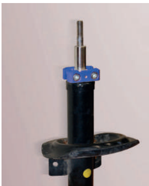
Position the clamp with the fixing screws. Do not tighten.
