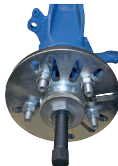
Drive shaft extraction from hub
