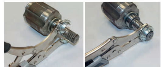
Clamps come down automatically when the joint opens. Ideal for saving the axle shaft without risking damage and having to replace it completely.
