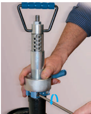
When the removal is completed, lock the clamp with the screws.
